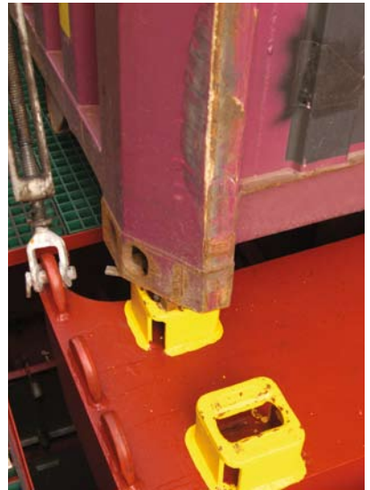
CORNER CASTING ARRANGEMENT FOR A EURO CONTAINER
