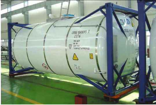
TYPICAL ARRANGEMENT FOR A TANK CONTAINER
